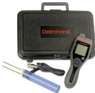
Pin-type moisture meter, Delmhorst BDX-20
